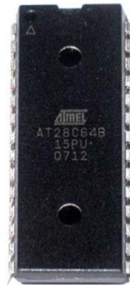
8 KB (64 Kbit) EEPROM AT28C64B (Atmel)
