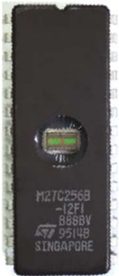
32 KB (256 Kbit) EPROM M27C256B (ST Microelectronics)
